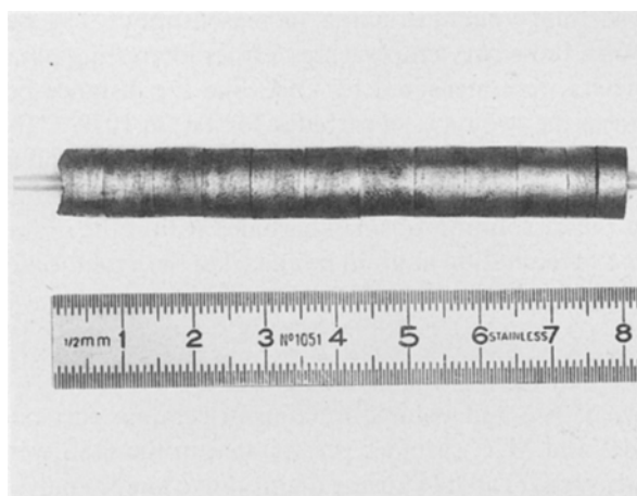
Figure 2 Optical image of a sintered pile of samples (M3/2 + 7 wt % \text{Cu}_3\text{P} + 0.25 wt % C) + 10 vol % TiC.
